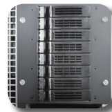
8 x 2.5" HDD cage with mini-SAS backplane
